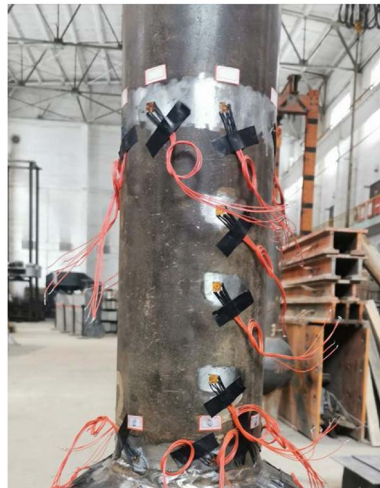
Figure 2. Physical drawing of steel pipe measuring point arrangement 图 2. 钢管测点布置实物图
