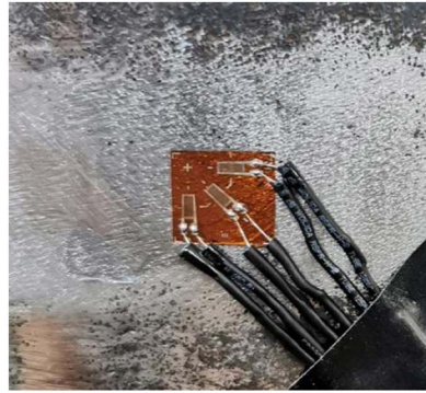
Figure 5. Schematic diagram of three-way strain flower
