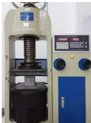
Figure 2. Cube compressive strength test device 图 2. 立方体抗压强度试验装置
