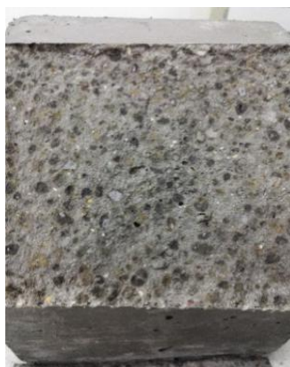
Figure 3. Internal properties of the specimen at failure 图 3. 破坏时试件内部性状
