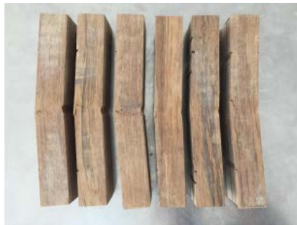
Figure 4. Test piece after shear failure
