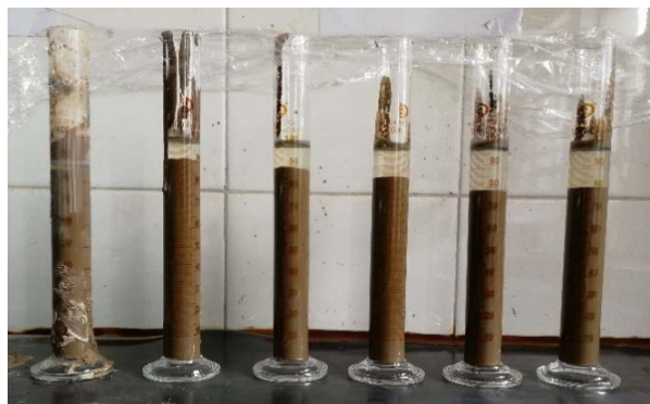
Figure 4. Stability test of mixed mud 图 4. 混合泥浆稳定性试验
