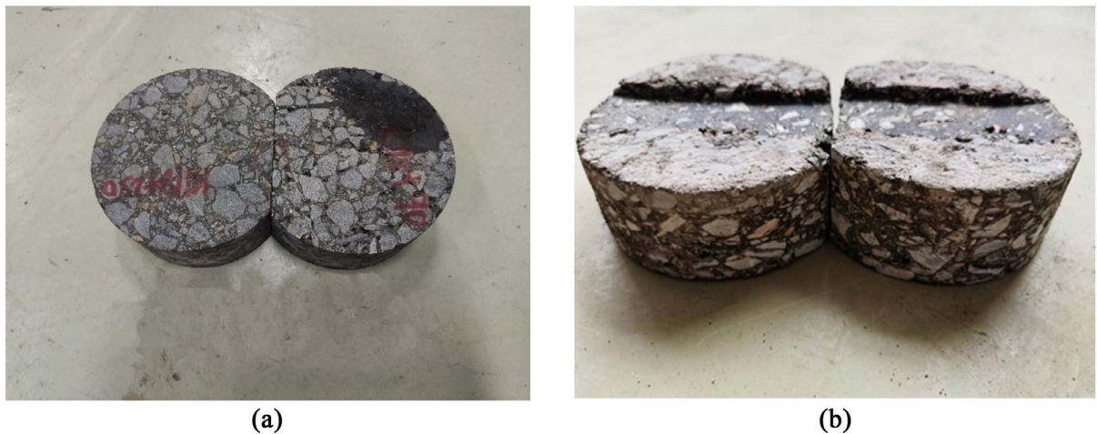
Figure 12. Comparison of Hamburg rutting test before and after. (a) Hamburg rut specimen before test; (b) Hamburg rutting specimen after test
