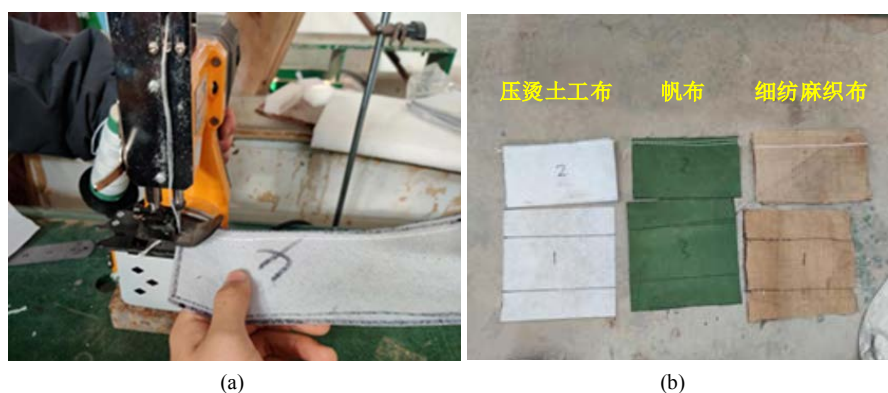
Figure 1. The sewing process of the geotextile and the samples used in the tensile strength test. (a) The sewing process of the geotextile (b) The test samples
