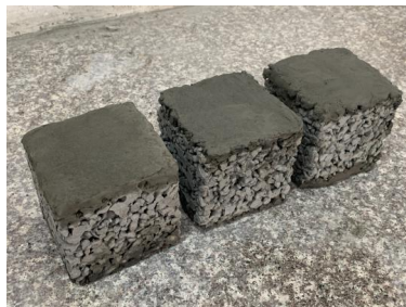
Figure 2. Cement paste to smooth the compressive test block 图 2. 水泥净浆抹平的抗压试块
