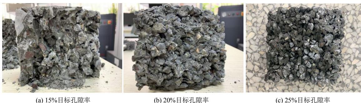
Figure 8. Fracture section of pervious concrete under three goal porosities with 6% silica fume 图 8. 硅灰掺量为 6% 时三种目标孔隙率下透水混凝土的破坏断面
