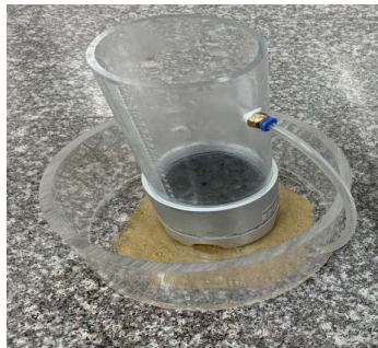
Figure 4. Permeability coefficient testing device 图4. 透水系数测试装置
