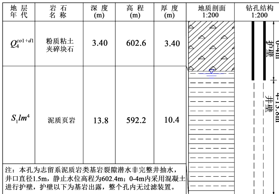
Figure 4. Profile characteristic map of dewatering well in site area 图 4. 场区降水井剖面特征图
