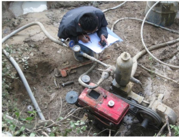
Figure 3. Slope water pressure test site 图 3. 边坡压水试验现场图
