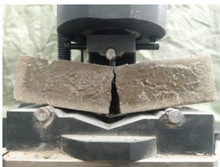
Figure 1. Flexural strength test device
