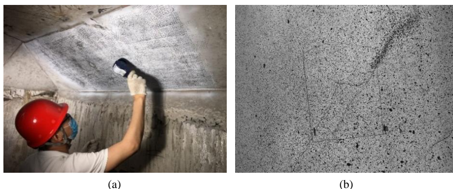
Figure 2. Fabrication of box beam scattered spot. (a) Box beam large field of view scattered spot map; (b) Box girder small field of view scattered spot map
