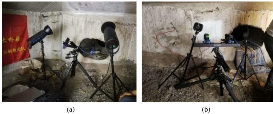
Figure 3. Test system arrangement. (a) Box girder full field system arrangement; (b) Box girder local system arrangement
