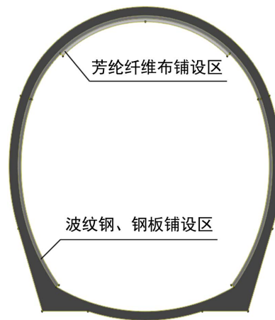
Figure 4. Schematic diagram of laying range of reinforced structure 图 4. 加固结构铺设范围示意图
