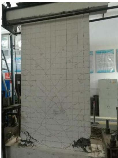
Figure 2. Final failure state of test piece 图 2. 试件最终破坏状态
