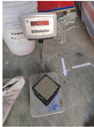
Figure 1. Test of bulk density of all light ceramsite concrete 图 1. 全轻陶粒混凝土容重测试
