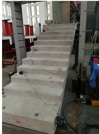
Figure 5. Test device drawing for stair performance 图 5. 楼梯性能试验装置图
