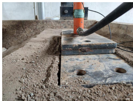
Figure 11. The surface of the fill collapsed 图 11. 填土表面塌陷
