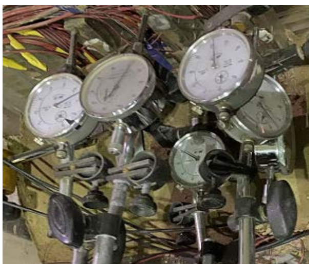
Figure 11. Pile body dial gauge arrangement
