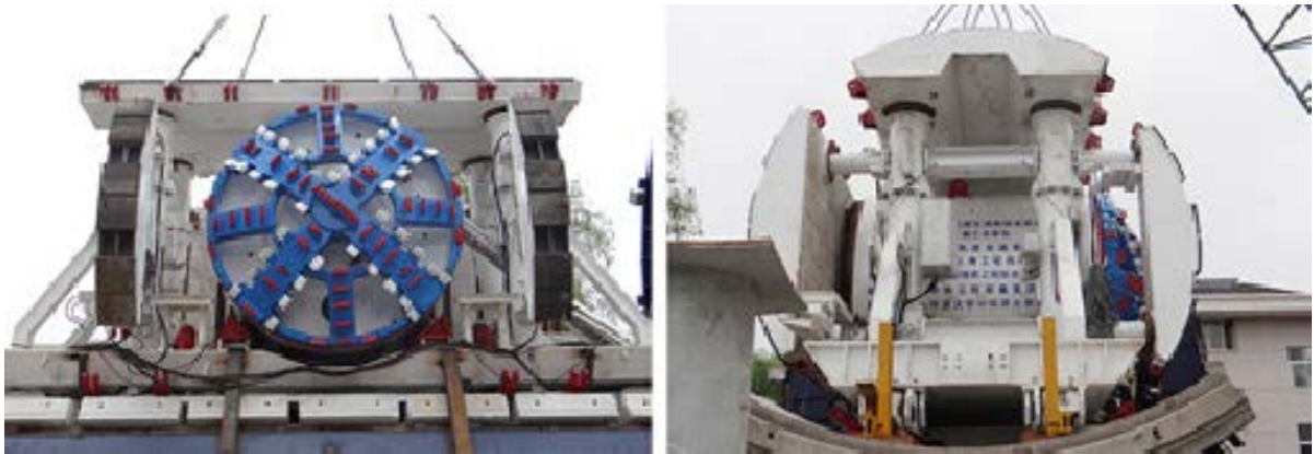
Figure 1. Mobile segment prestressing support system 图 1. 移动式管片预应力支撑系统
