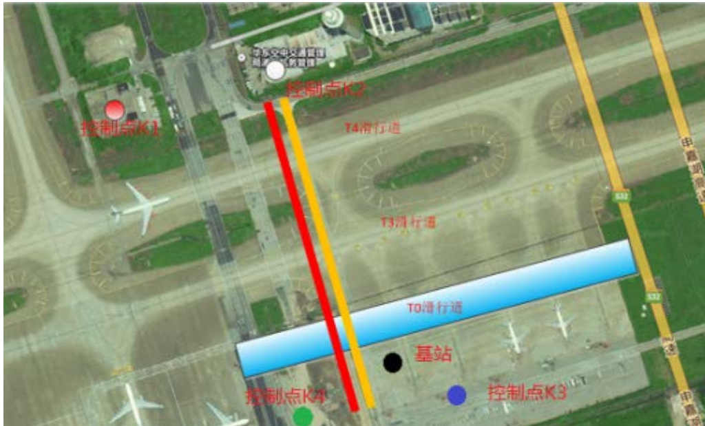
Figure 3. Layout plan of base station and control points 图 3. 基站和控制点布设平面图
