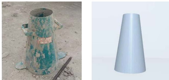
Figure 2. Slump test equipment 图 2. 坍落度试验设备
