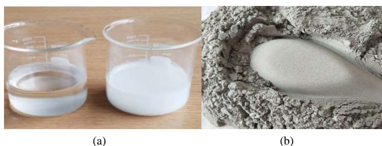
Figure 1. Test materials: (a) Paraffin based phase change materials; (b) Fly ash
