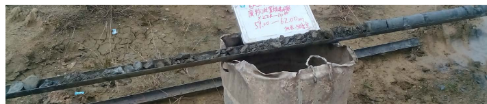
Figure 8. Photo of fault fractured zone exposed by borehole XZZK10 图 8. 钻孔 XZZK10 揭露断层破碎带照片
