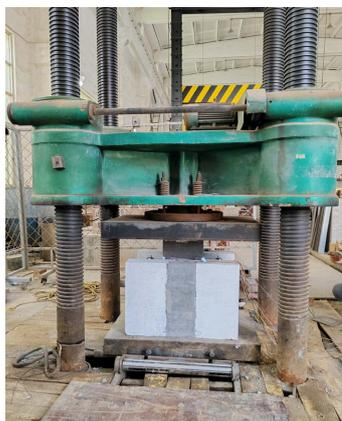
Figure 2. Loading device diagram of the push-out specimen
