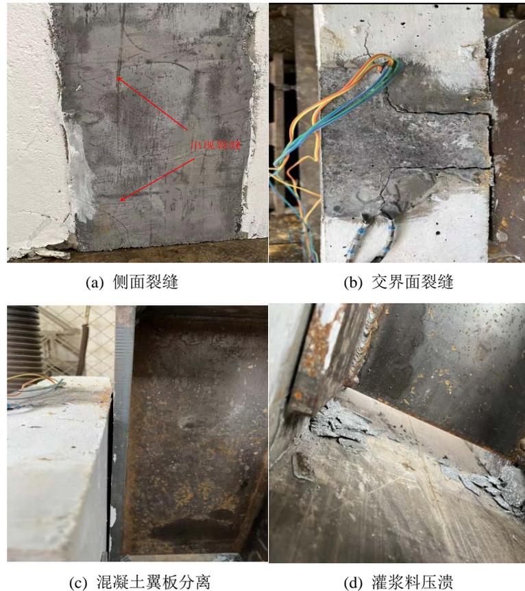
**Figure 4.** The failure modes of the specimen: (a) Side cracks; (b) Interface cracks; (c) Separation of concrete wing plate; (d) Grouting material crushing
