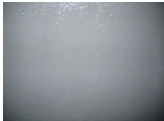
Figure 2. Part photo of glass flake after sealing 图 2. 玻璃鳞片封闭后局部照片
