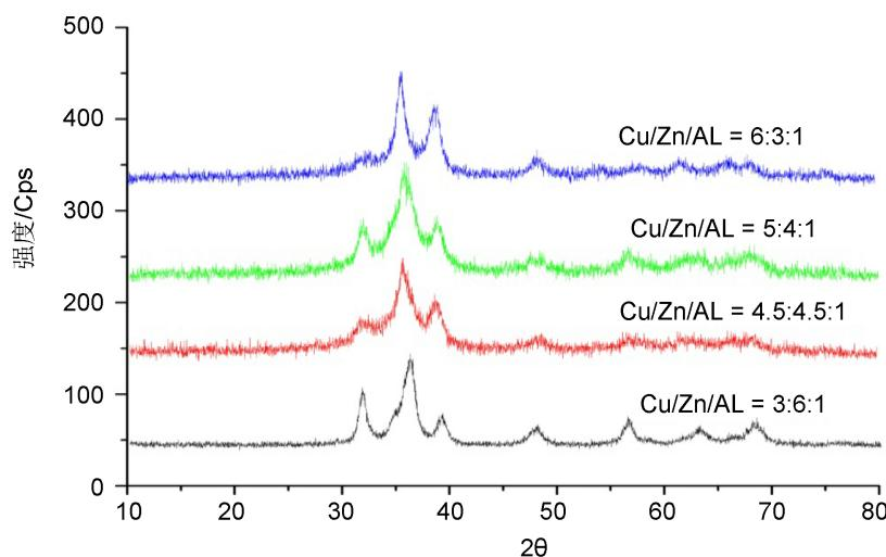
**Figure 1.** XRD of catalysts with different ratios of Cu/Zn/Al
