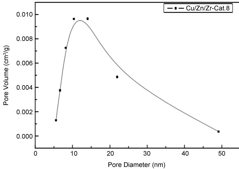
**Figure 3.** Distribution curve of pore size
