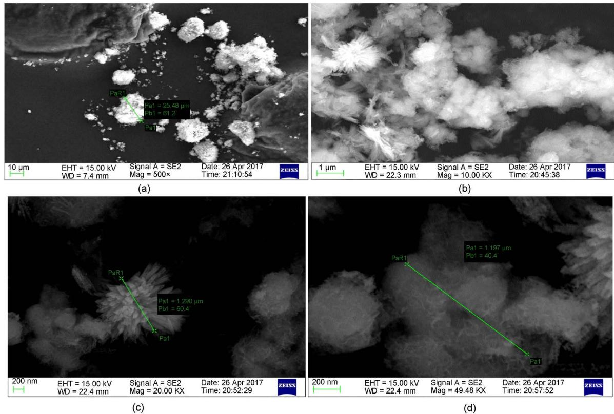
**Figure 4.** SEM image of catalysts with Cu/Zn/Al = 4.5:4.5:1
