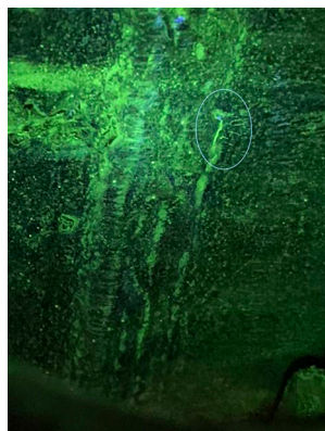
Figure 4. The inner-surface crack detected by magnetic particle examination
