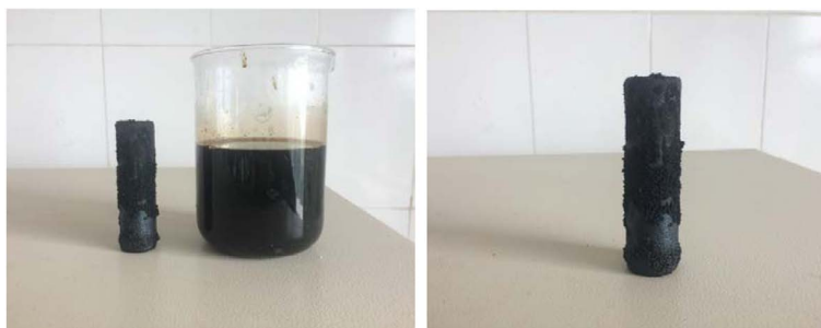
Figure 1. D56 cores immersed in temporary plugging liquid at 150°C for 7 days
