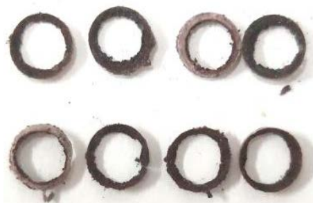
Figure 7. Images of the remaining residues of combustion of HMX/graphite/Fe 2 O 3 composite energetic materials
