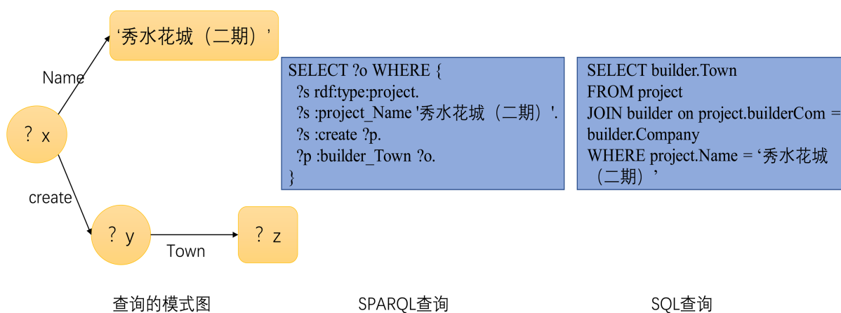
Figure 4. SPARQL converted to SQL instance
