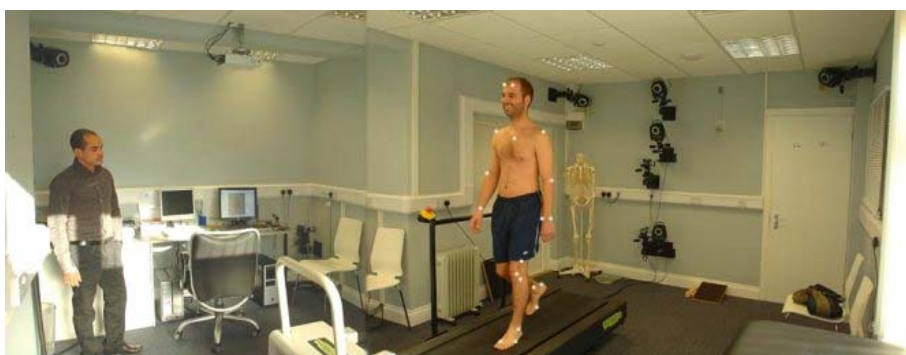
Figure 3. The 3D gait analysis system is in the work 图 3. 示三维步态分析系统在工作
