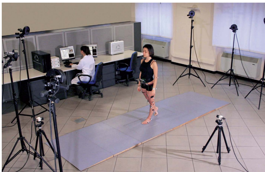
Figure 3. The 3D gait analysis system is in the work 图 3. 示三维步态分析系统在工作
