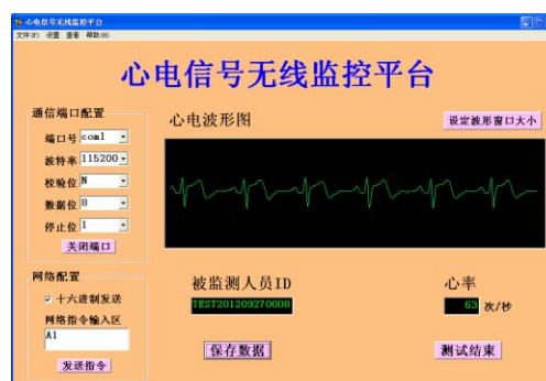
Figure 7. Experiment result of wireless ECG sensor node 图 7. 无线心电传感器节点测试实验结果
