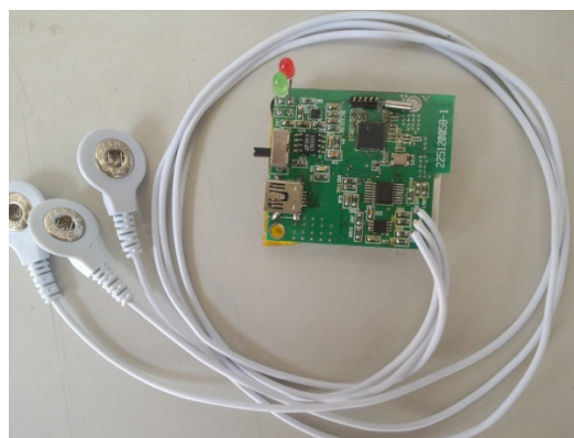
Figure 4. Picture of wireless ECG sensor node 图 4. 无线心电监测传感器节点实物图
