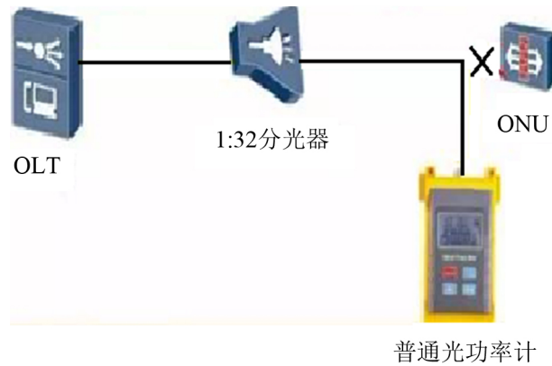
Figure-2. Using ordinary optical power meter for down light power test
