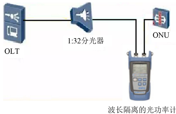
Figure 3. Optical power meter with wavelength separation for bidirectional optical power test
