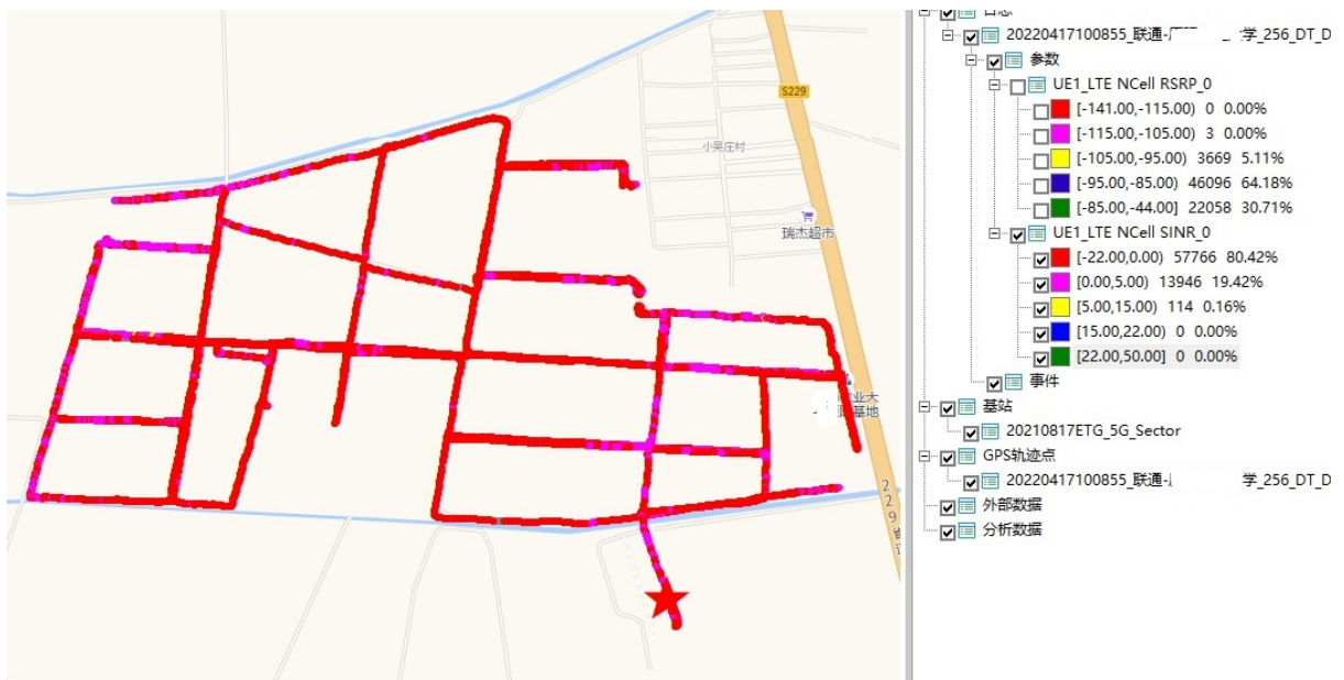
Figure 2. 4G signal to interference plus noise ratio 图 2. 4G 信号与干扰加噪声比
