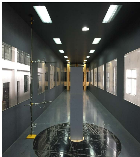
Figure 2. Model in the wind tunnel
