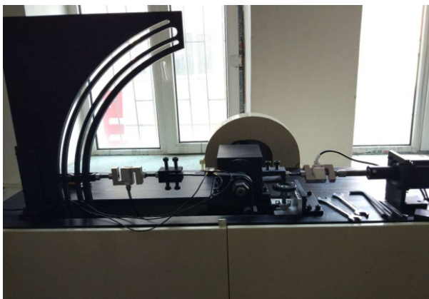
Figure 4. Multi-wedge friction coefficient testing bench 图 4. 多楔带摩擦系数测试试验台
