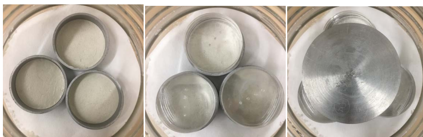
Figure 18. Soil sample placement and top loading
