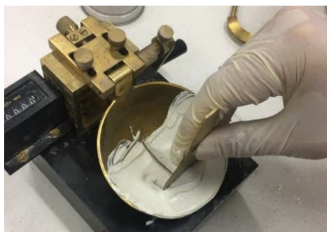
Figure 1. Liquid limit determination process
