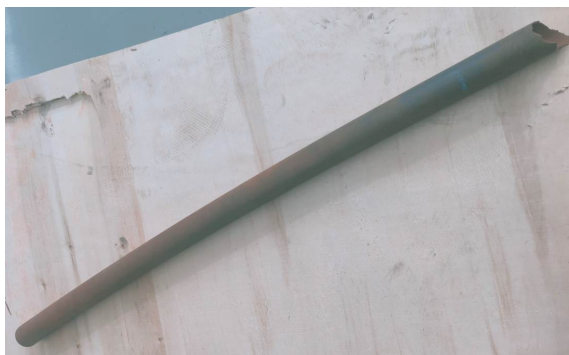
Figure 1. Coiled tube with fracture
