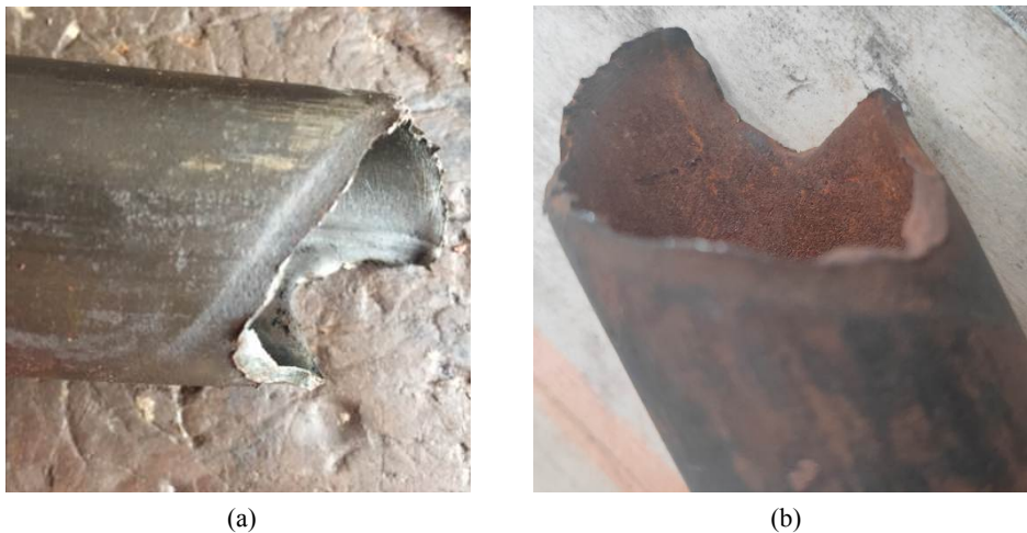
Figure 3. Fracture morphology of coiled tube. (a) Failure scene morphology; (b) Morphology in laboratory 图 3. 失效连续油管断口形貌。(a) 失效现场形貌; (b) 实验室形貌
