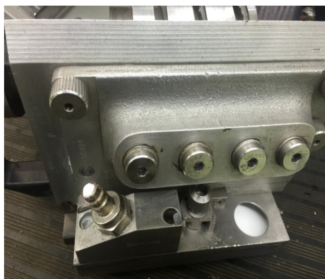
Figure 6. The trademark glue cylinder before add lining 图 6. 增加内衬管前的商标胶缸
