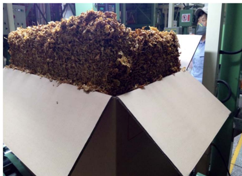
Figure 2. The smoke sheet expands above the opening of the smoke box
