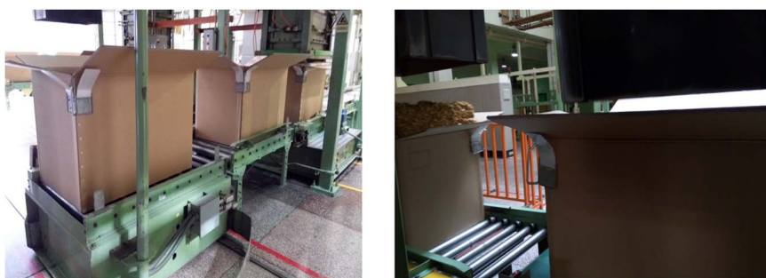
Figure 9. Installation diagram of reset device supported by cover plate of smoke box 图9. 烟箱盖板支撑复位装置安装图
