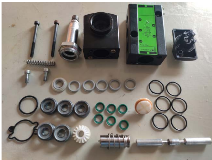
Figure 5. Components of solenoid valves
