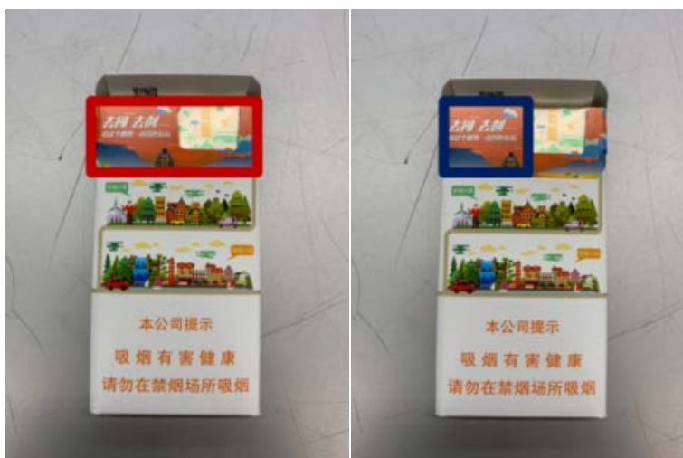
Figure 7. Select the missing paper detection retrieval area and the template area 图 7. 选择缺卡纸检测检索区域以及模板区域
