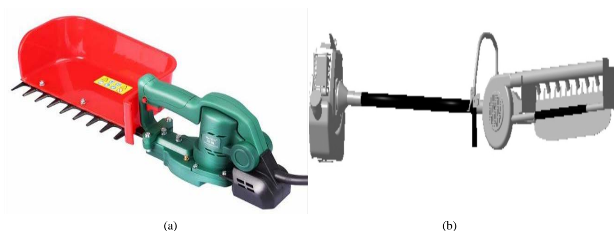
Figure 1. (a) Single person electric tea picking machine; (b) Single person knapsack tea picking machine 图 1. (a) 单人电动采茶机; (b) 单人背负式采茶机
