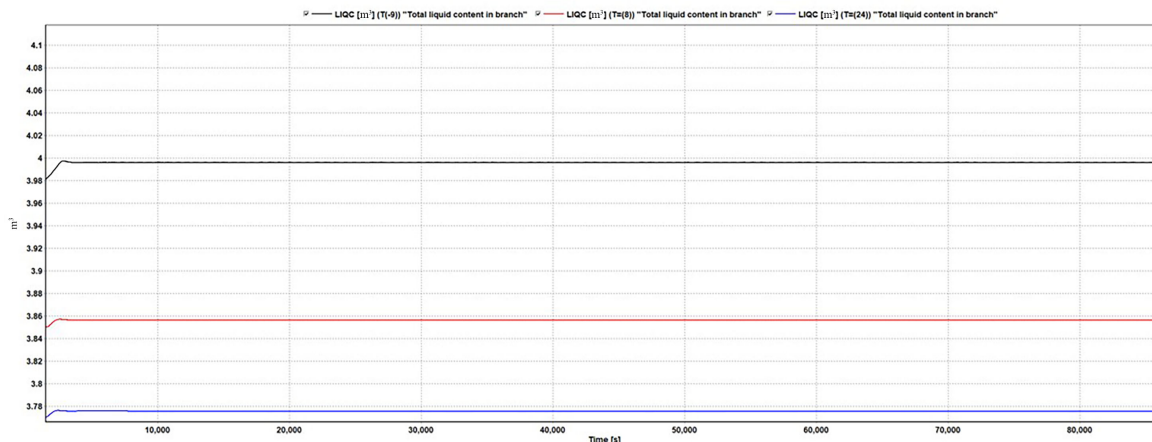
Figure 12. Total liquid accumulation in pipelines under different ambient temperatures ( -9^{\circ}\text{C} , 8^{\circ}\text{C} , 24^{\circ}\text{C} )
