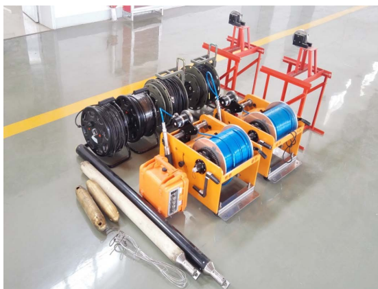
Figure 2. Physical object of magnetic antenna CT 图 2. 磁天线 CT 实物图
