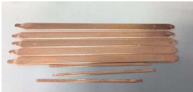
Figure 11. Schematic diagram of flat channel heat pipe 图 11. 扁平化槽道热管示意图
