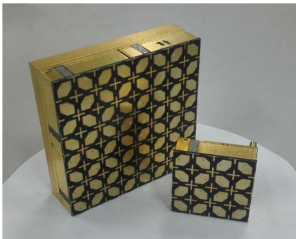
Figure 7. Multichannel tile-type on-chip antenna
