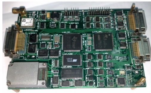
Figure 1. Flight control board-gyro data acquisition platform 图 1. 飞控板-陀螺仪数据采集平台
