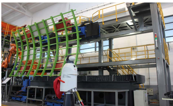
Figure 2. The on-site measurement of laser tracker 图 2. 激光跟踪仪现场转站测量
