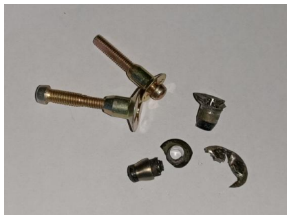
Figure 5. Comparison of normal rivets and rivet remains 图 5. 正常铆钉与铆钉残骸对比
