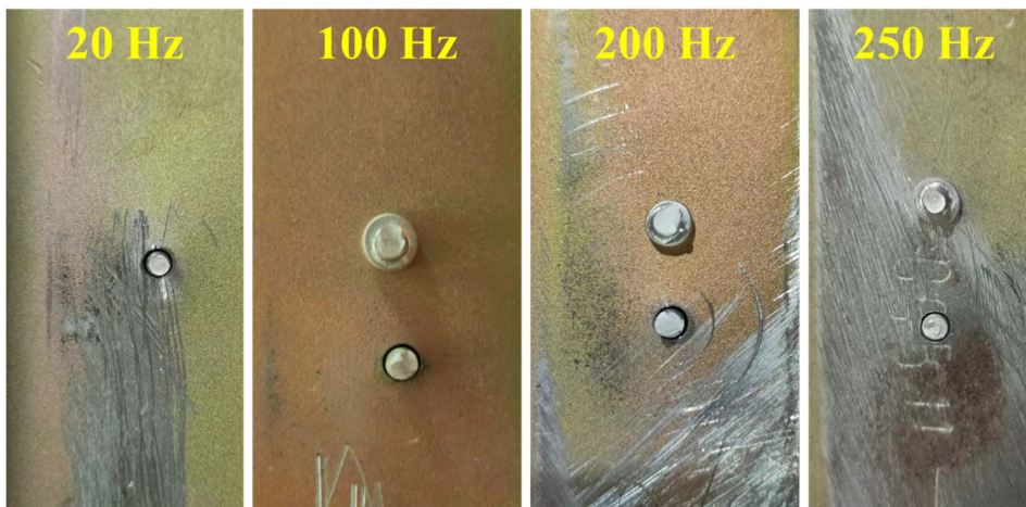
Figure 5. Fatigue failure diagram of aircraft riveted joints 图 5. 飞行器铆接接头疲劳失效图
