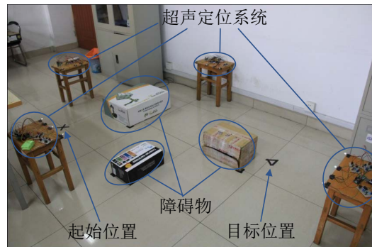
Figure 16. Obstacles set in the indoor simulation experiment
