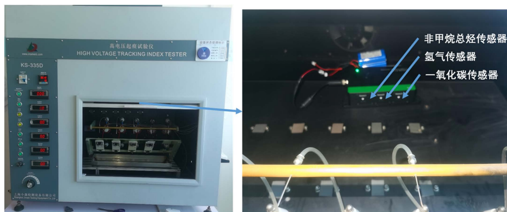
Figure 4. Electric tracking process gas detection device
