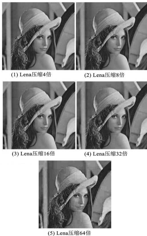
Figure 2. Compression Lena graph based on dual density dual tree complex wavelet transform 图 2. 基于双密度双树复小波变换压缩 Lena 图
